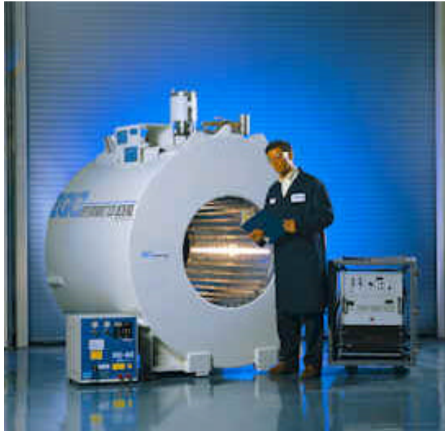
Figure 6: IGC 1.5T active shielded MRI magnet.
