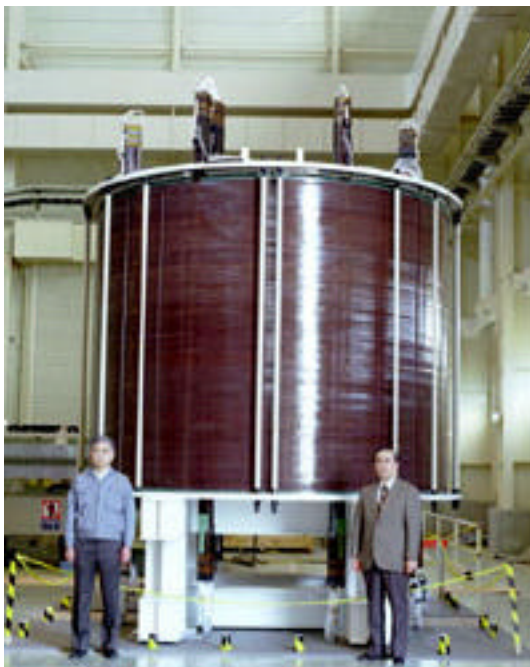
Figure 12: 13T CSMC test coil and cutaway view of assembly.
