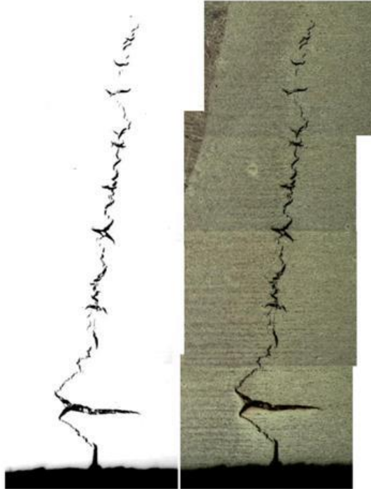
Figure 2. Microstructural features of SOHIC.
