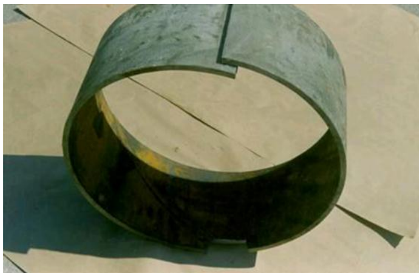
Figure 3. Residual Stress, a “Critical Factor” – cut section of linepipe exhibiting displacement due to residual stress.
