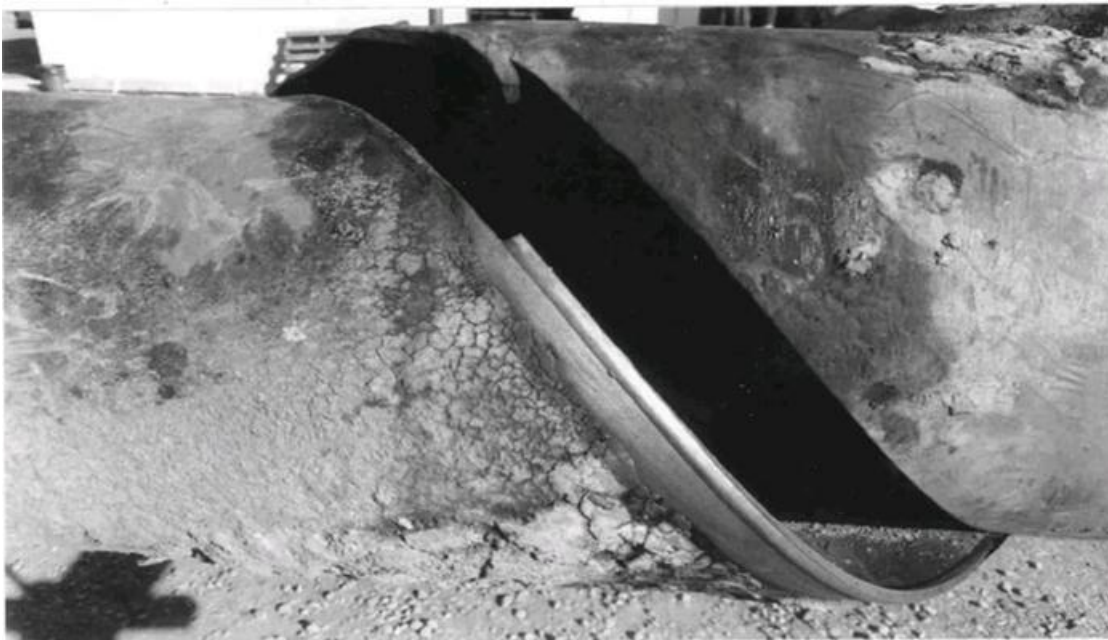
Figure 1. SOHIC failure of spiral welded pipe, courtesy Shell Canada.
