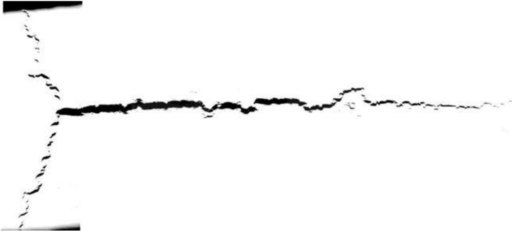
Figure 5. SOHIC in a dished end.
