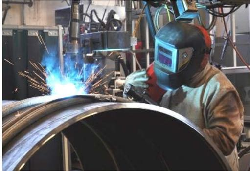
Figure 18. Weldability assessment of X80 HTS pipe segments (GMAW - 1G position).
