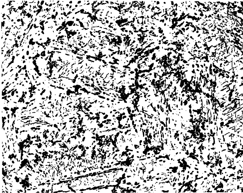
M 3 C Carbides in the Mo-Cb-Modified AISI 4130 Steel
