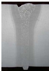
Figure 8. RPEB weld in 25 mm thick plate.
