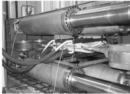
Figure 18. Wide plate specimen with cooling boxes in the 8000 kN tensile testing rig.
