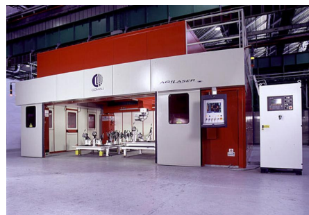
Figure 25. Assembly technologies: the Comau Agilaser laser welding solution.
