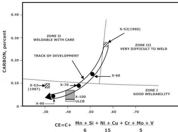
Figure 1. “Weldability Diagram” according to Graville [3].
