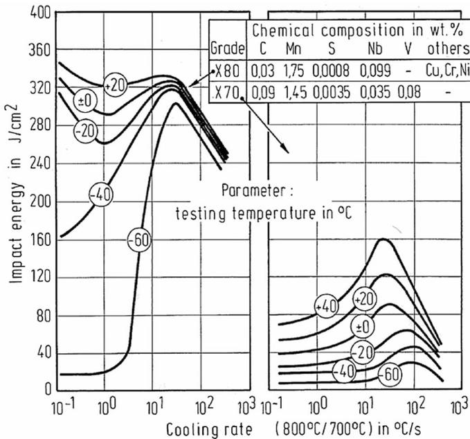
Figure 2. Comparison of HAZ toughness of conventional 0.09 percent carbon Nb-V steel and 0.03 percent carbon HTP (High Temperature Processed) steels in simulation tests [5].
