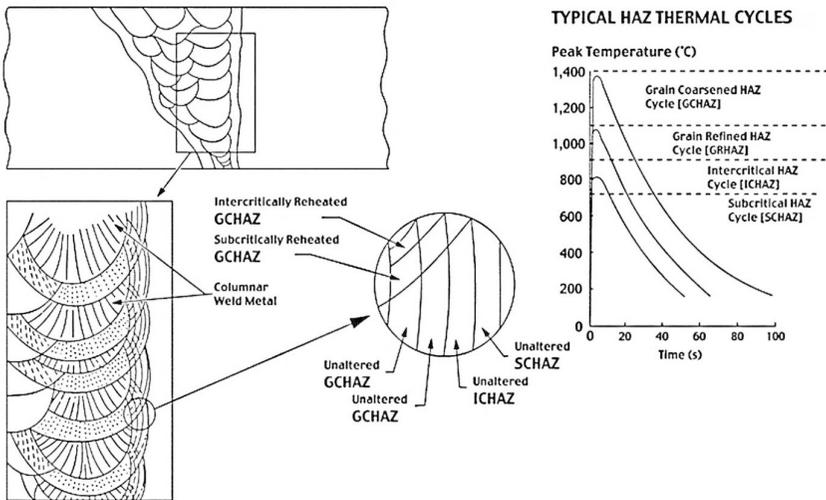
Figure 6. Range of overlapping thermally cycled regions in the weld HAZ [9].
