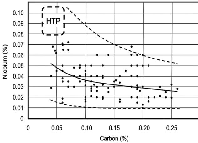
Figure 15. Combinations of niobium and carbon contents in operating pipelines in N. America, and UK circa 1977 [24, 27].
