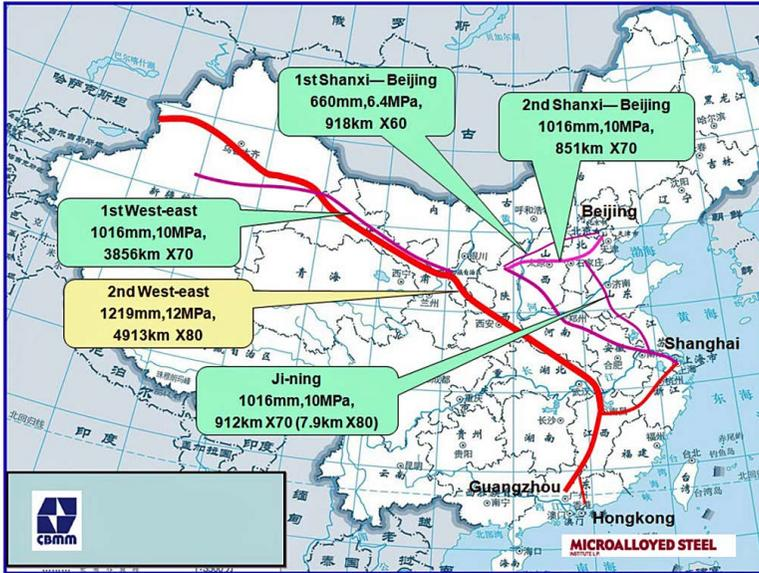
Figure 17. Map showing the Second West East Pipeline built by CNPC.
