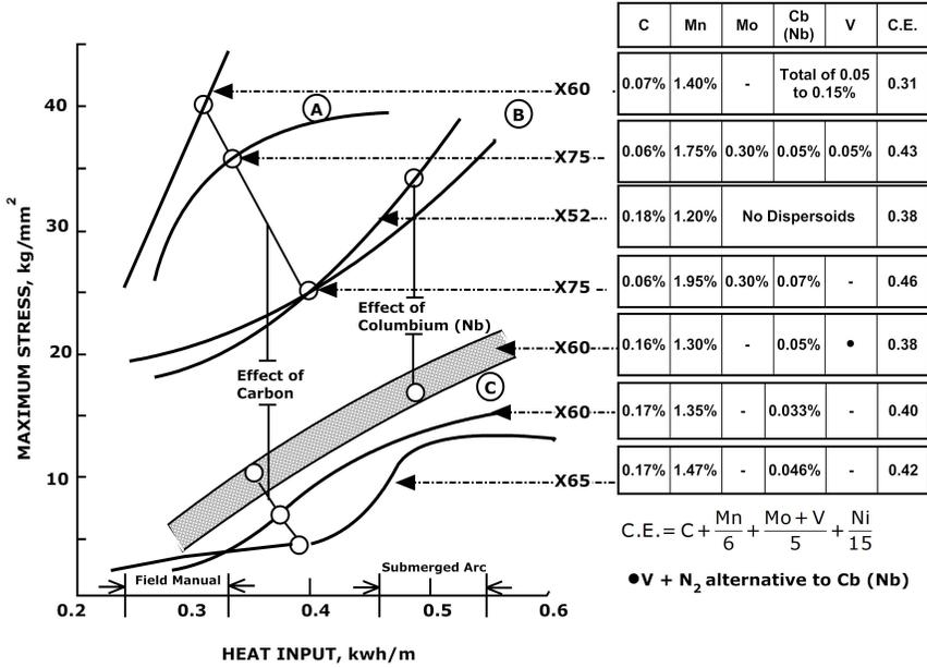
Figure 4. Implant test results for steels with various carbon contents [7].
