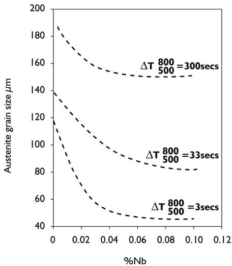
Figure 11. Effect of niobium content and cooling rate on austenite grain size in the HAZ [18].
