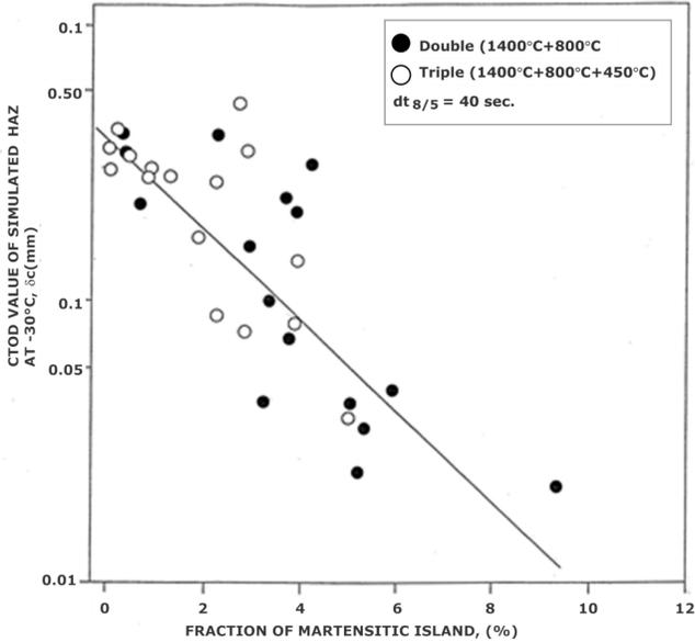
Figure 9. Effect of MA content on HAZ CTOD toughness in simulated welds [16].
