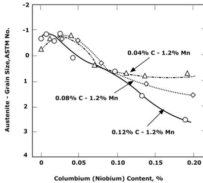
Figure 12. Austenite grain coarsening behaviour for steels reheated to 1200 °C for 1 hr and water quenched [19].
