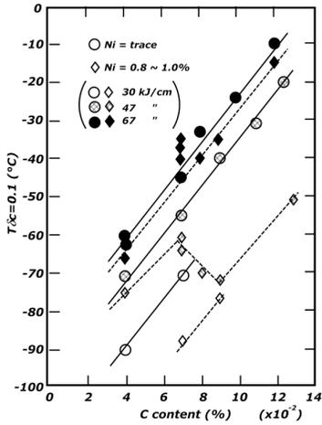
Figure 3. Effect of carbon content on HAZ Charpy V-notch transition temperature [6].
