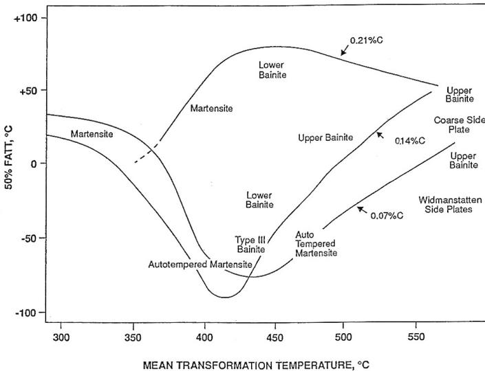
Figure 7. Effect of carbon content, and mean transformation temperature on HAZ 50 percent shear transition temperature [12, 13].
