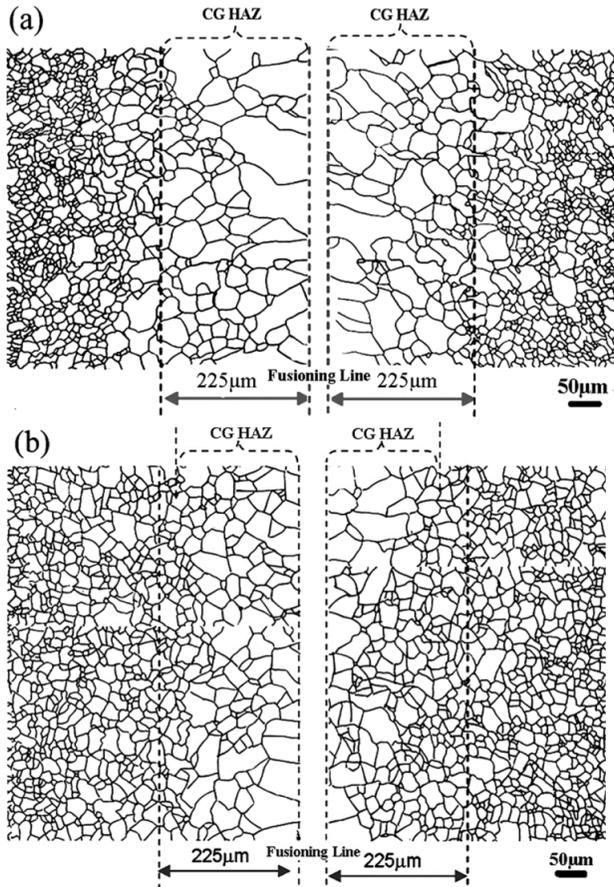
Figure 18. Distribution of prior austenite grains in actual HAZ (a) medium Nb steel (0.05 wt%); (b) higher Nb steel (0.09 wt%) [26].
