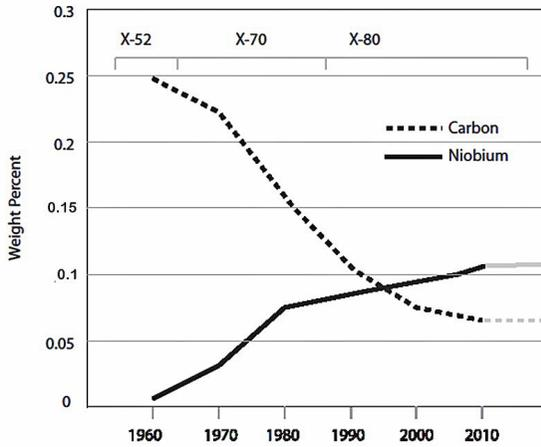
Figure 16. Changes in maximum niobium and carbon contents with time (and strength increase).
