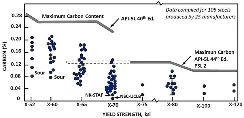
Figure 5. Trend of carbon content with pipe yield strength [8].
