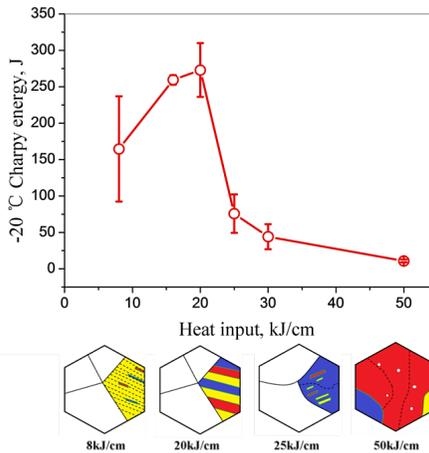
Figure 13. Density of high angle (> 45°) boundaries associated with high and low toughness microstructures [14].
