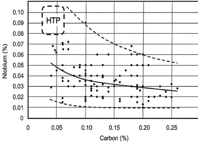
Figure 15. Combinations of niobium and carbon contents in operating pipelines in N. America, and UK circa 1977 [24, 27].
