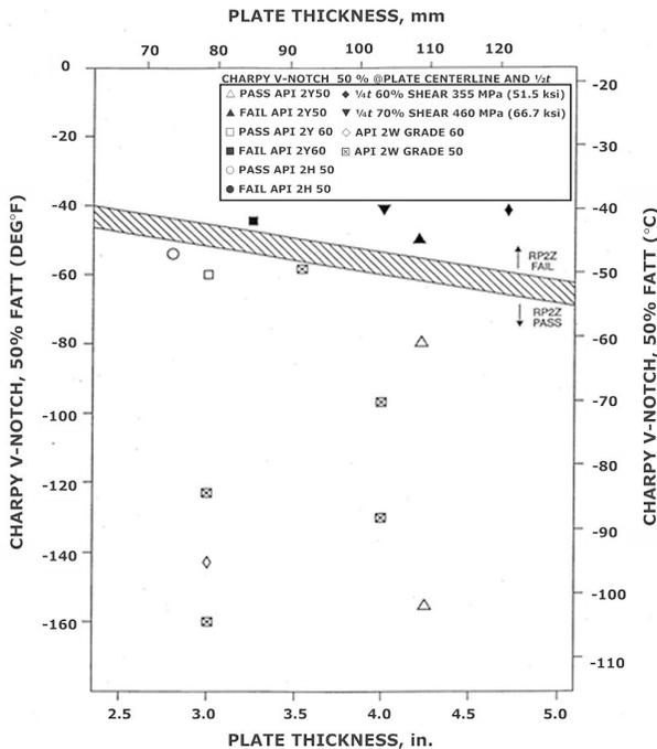
Figure 14. Effect of unwelded Charpy FATT on successful outcome of API RP2Z Prequalification Testing.
