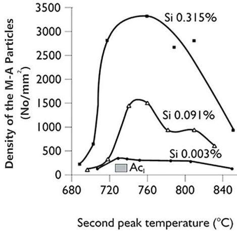
Figure 10. Effect of silicon on proportion of MA phase (Aspect Ratio>4; Lmax>2 $\mu$ m) in reheated HAZ regions [17].
