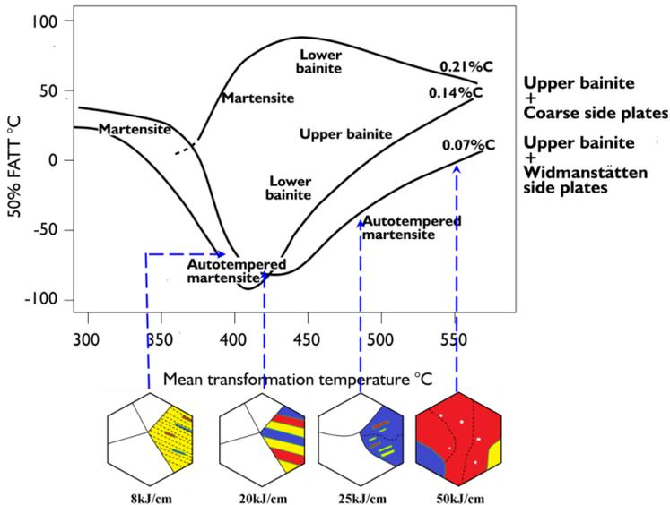
Figure 8. Range of microstructures associated with regions of high and low HAZ toughness[11].
