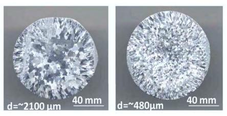
Extensive research showed Niobium to significantly reduce the grain size in AlSi alloys over industry established Titanium grain refiner.
