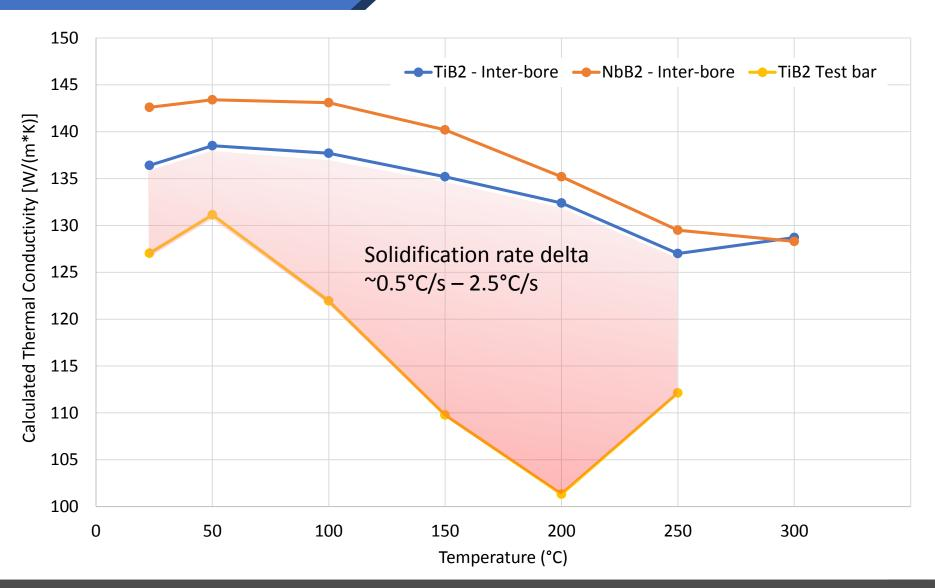
Thermal conductivity was calculated using the thermal diffusivity, density, and heat capacity of the material.
