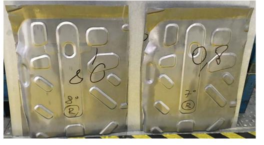
The cold formed panels were been heat treated and assembled as archetypes of the standard floors
