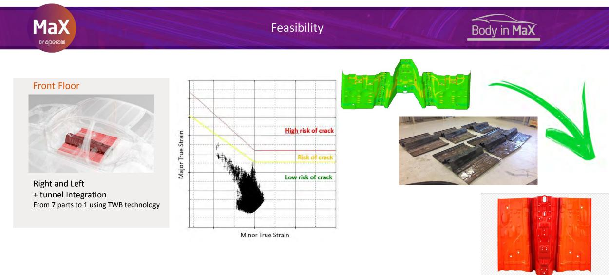
More and more manufacturers are using hot stamping parts. We propose the innovative concept of joining a low thickness part and a TWB. By taking advantage of reinforcement integration, only one part needs to be produced.
