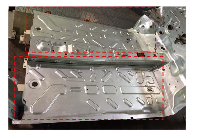
Floor panels cold stamped with standard DP600 0,8 mm thickness
