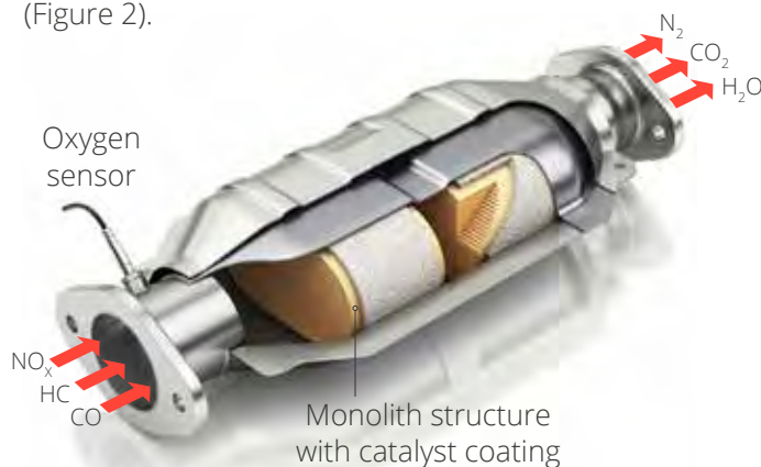
Figure 2. Three Way Catalytic Converter.
