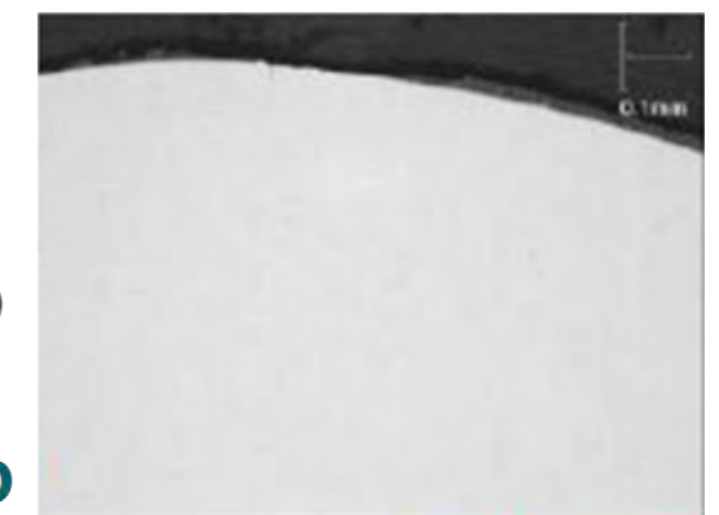
Top of the 3rd layer after IG corrosion test (with bending)
