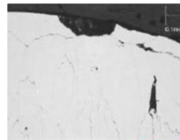
Top of the 3rd layer after IG corrosion test (with bending)
