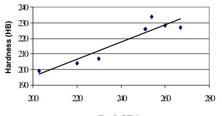
**Tensile (MPa)** Figure 3: Hardness versus tensile strength
