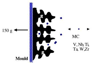
Figure 5: Schematic illustration of the solidification in a spin casting mould.
