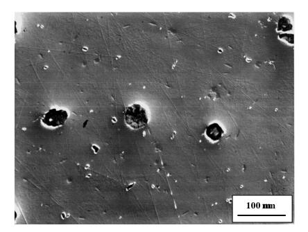
Figure 4: Nodular iron roll material with additions of niobium showing small discrete NbC particles homogeneously distributed in the structure.
