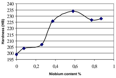
Figure 2: Hardness (HB) as a function of niobium content.
