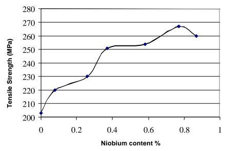
Figure 1: Tensile strength (MPa) as a function of niobium content.
