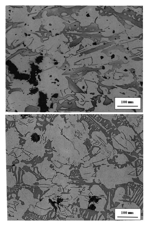
Figure 7: Some example of microstructure of carbide reinforced IC material.
