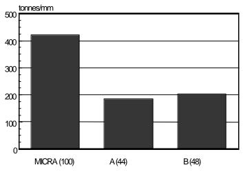
Figure 9: Performance of MICRA rolls in a Steckel mill.
